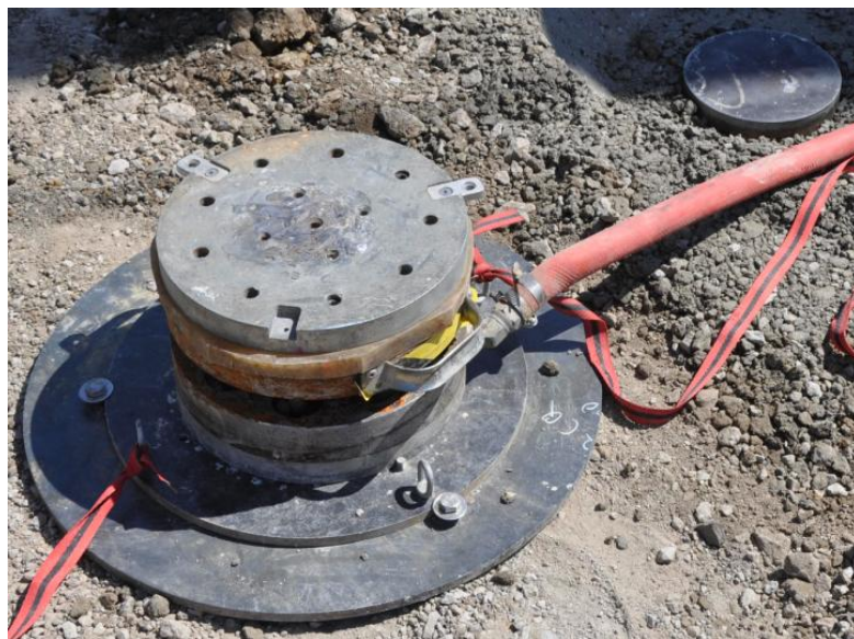
Figure 23. The RAM Test in the field with the 9 in. steel plate in the upper right corner, and the 18 in. and 24 in. plates attached to the device
